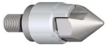
Completely Fixed Valves: these are generally considered ball-check valves. The entire valve is fixed to the feed screw flow through channels on the inside of the valve with a ball or pin to control flow.
