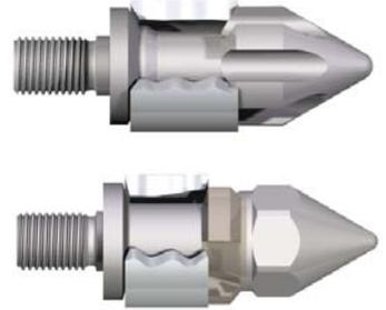
Floating & Fixed Rotation Check Rings: these valves have check rings with feet or pins that lock the ring into the rotation of the feed screw, often referred to as "locking check rings". The ring still has lateral freedom of movement.
