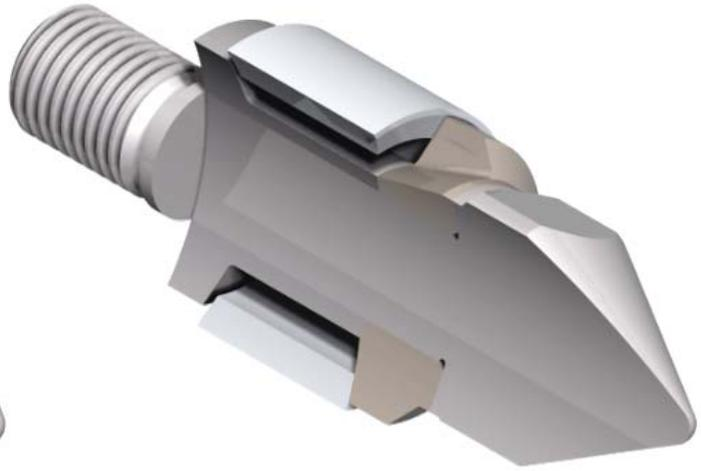
The design offers excellent wear resistance on the main replaceable wear components – the ring, wear seat and rear seat. These are combined with an extremely high tensile strength retainer (stud) to withstand shock or rigors of improper starting.
