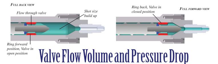
The key element in a screw tip valve is the flow volume through the valve. Higher flow volumes are generally referred to as Free Flow Designs; many ball check and some hybrid 3 and 4-piece construction designs offer very limited flow areas. Flow volumes are both a function of mechanical limitations and functionality needs. Common designs generally have flow volumes that range from 35 to 75% of the cross section of the feed screws exit or meter area.
