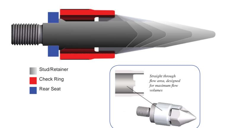
All three components of the P-770 Spin-Lock screw tip are manufactured from H-13 tool steel that is heat-treated to the maximum safe Rockwell hardness, based on the valve geometry that will range from 52 to 59. The components are Ion Nitride surface hardened for added wear protection. Nitride provides a case hardness of up to 70 Rockwell with a case depth of up to .015" per side.
