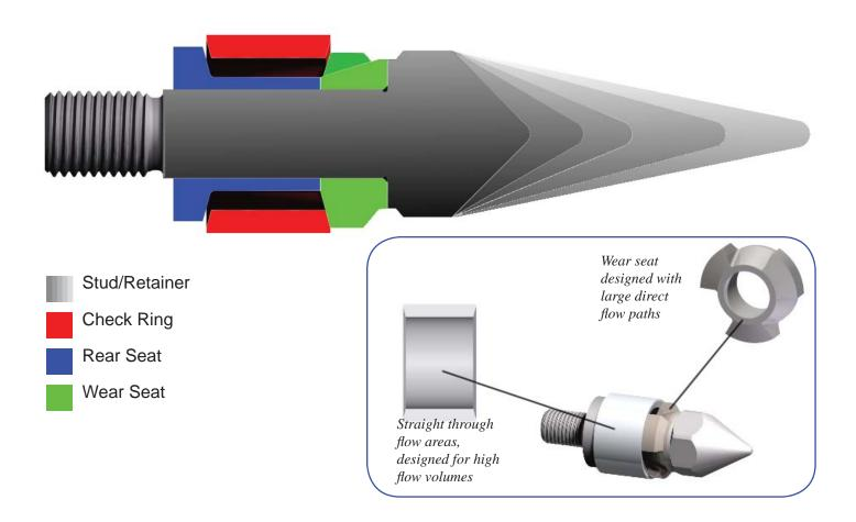
The key wear components are manufactured from high quality tool steels containing very high levels of the carbide forming element Vanadium which is one of the hardest and most wear resistant carbides.
