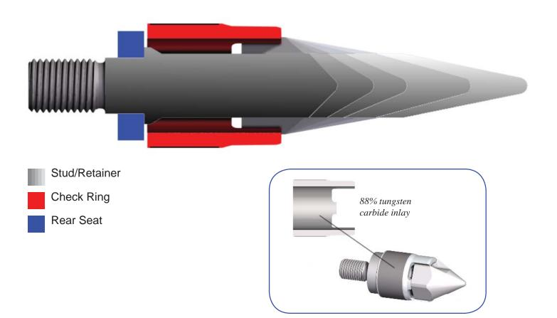
The screw tip (stud) and rear seat are manufactured from H-13 tool steel that is heat-treated to the maximum safe Rockwell hardness, based on the valve geometry that will range from 52 to 59. The components are Ion Nitride, surface hardened for added wear protection. Nitride provides a case hardness of up to 70 Rockwell with a case depth of up to .015" per side.
