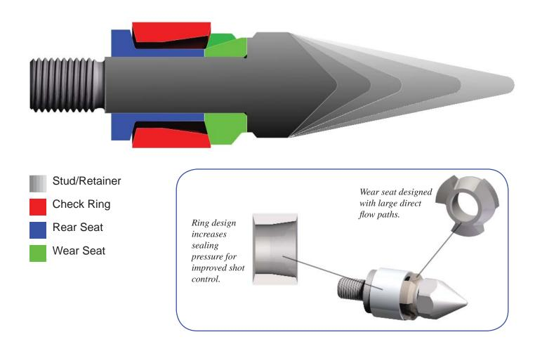
The key wear components are manufactured from high quality tool steels containing very high levels of the carbide forming element, Vanadium, which is one of the hardest and most wear resistant carbides.
