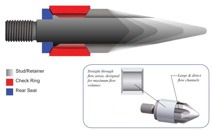
All three components of the P-700 screw tip are manufactured from H-13 tool steel that is heattreated to the maximum safe Rockwell hardness, based on the valve geometry that will range from 52 to 59. The components are Ion Nitride surface hardened for added wear protection. Nitride provides a case hardness of up to 70 Rockwell with a case depth up to .015" per side.
