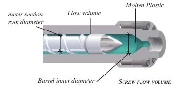
The more restrictive the flow requires the screw to build higher pressures and moves the areas of pressure buildup further back on the screw's length. This can be beneficial for some applications and materials that require greater energy for mixing action and present problems for other materials that are sensitive to shear or pressure energy.
